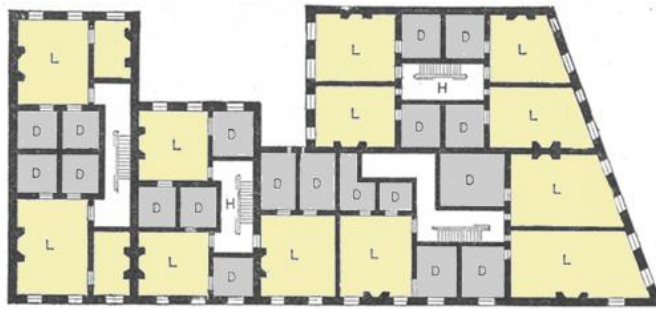
TENEMENT OF 1863. FOR TWELVE FAMILIES ON EACH FLAT 2 D. dark L. light H. halls.
