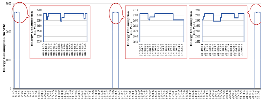
Figure 5. The energy consumption profile of geyser installed in kitchen.
