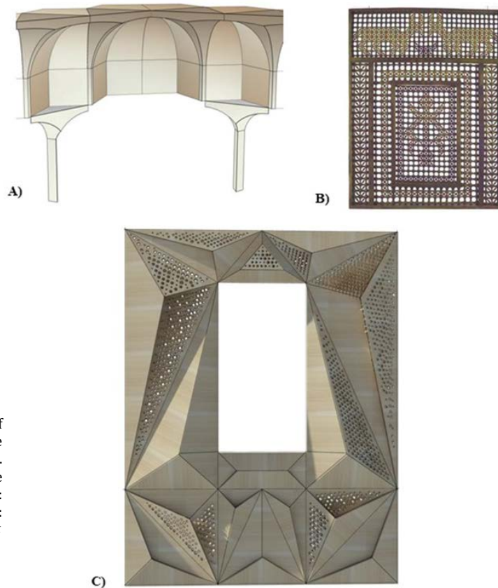
Figure 17. The process of designing the Adaptive Mashrabiya. A. 3D Muqarnas, B. Flat Mashrabiya, C. Adaptive Mashrabiya (Source for A and C: Authors. Source for B: https://www.meashots.com/photo/210117/wooden-latticed-window-(mashrabiya)-with-two-small-swinging-sash.html )
