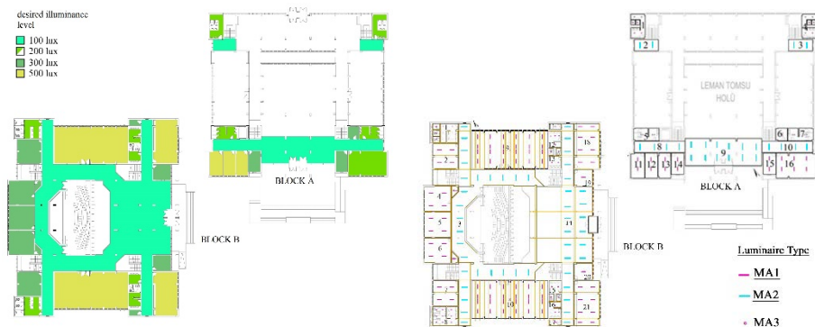
Figure 5. Ground Floor Plan and Existing Artificial Lighting Layout
