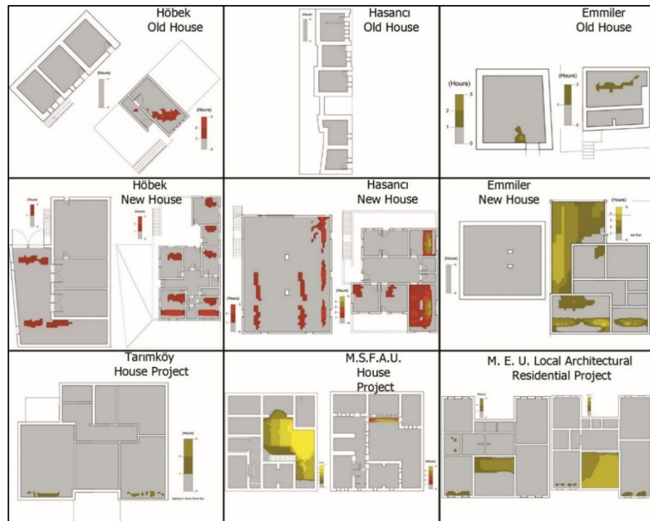
Figure 23. Direct daylight time analysis of selected houses.
