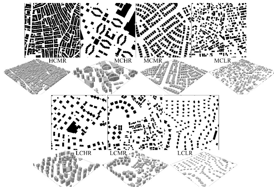
Figure 4. 2D/3D views from sample layouts of building typologies in UDM. Morphological form of long-linear building arrays in HCMR unfastens to distributed molecular form towards the LCLR typology.
