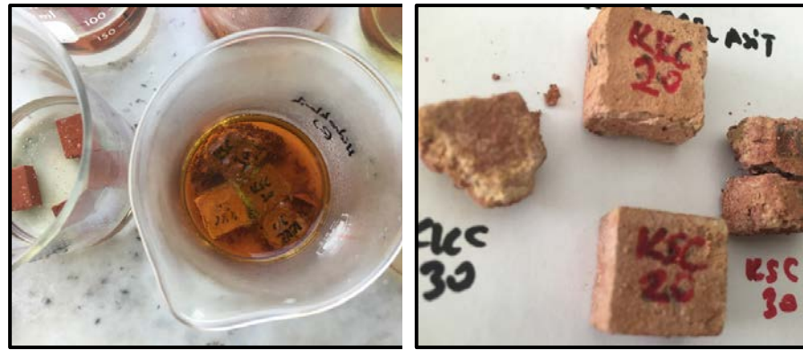
a. View of Samples in Hydrochloric Acid Bath
