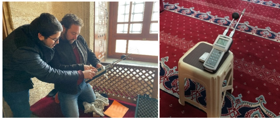
Figure 8. Hobo comfort analyser devices and D09847 climate analyser device were used in prayer halls on 21 st December. (In situ measurements) (Photographs by the authors, 2019).
