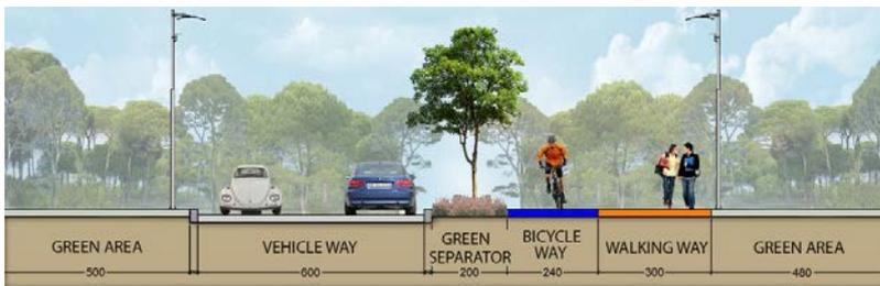
**Figure 4.** Recommended road section for the sustainable transport model (Demiroğlu et al., 2018).
