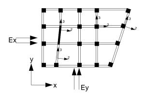
**Figure 12.** Non-orthogonal axis irregularity
