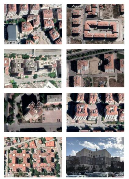
**Figure 8.** Several building layouts with projections in plan
