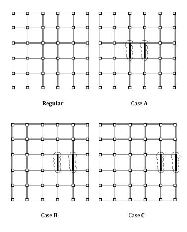
**Figure 18.** Models for analyzing the effect of shear wall location
