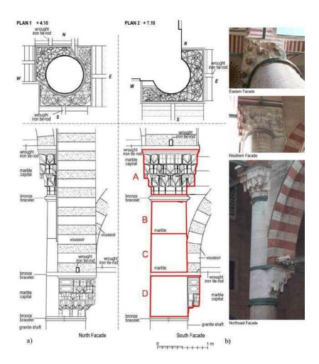
Figure 13. The CL1 column, Selimiye Mosque: a) scaled drawings of current state (drawn by Author) b) photographs, 2018 (Source: Author)
