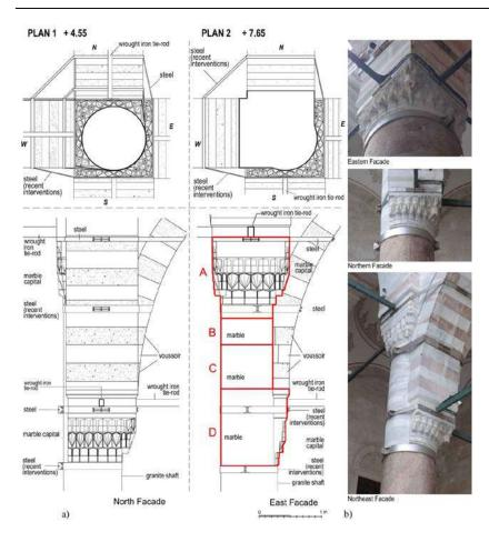
The building was recently repaired between 2007 and 2012. During this restoration, the column surface was cleaned, iron strains were cleaned and painted, and cracks were repaired by injection. The wrought iron tie-rods that lost their function were removed and a new stainless steel system was installed to strengthen the structure (Ceylan and Ocakcan, 2013; Çılı and Yıldız, 2013) (Figure 7a, b and 8).
