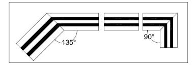
Figure 1. Slot Diffuser Linear and Corner Piece
