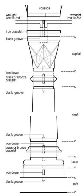
**Figure 4.** Schematic drawing of an ordinary column in Ottoman Classical Period (drawn by Author)
