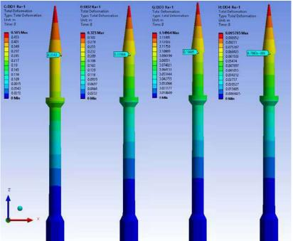
**Figure 7.** Top displacements of minaret model in case of DD-1, DD-2, DD-3 and DD-4 seismic hazard levels
