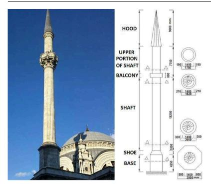
**Figure 2.** Photo (taken by author) and the dimensions of the minaret (Turk and Cosgun 2012)
