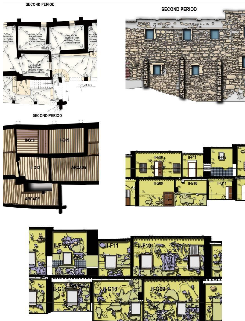
Figure 16. Detailed plan, sections, façade of second period
