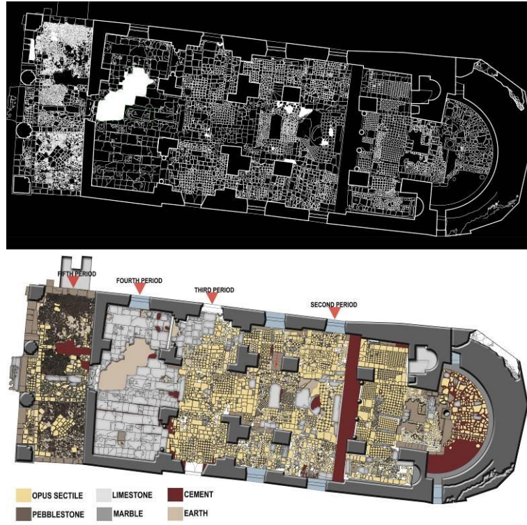
Figure 9. (a) Survey drawing of the church building, mosaics (b) analyses of the church building, mosaic stone types (c) image of the tombstone
