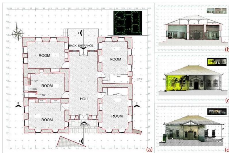
**Figure 8.** (a) Plan of building with exported points from Cyclone as dxf to Autocad. (b) One Section of Building. (c) South elevation drawing with ortho-images. (d) North elevation drawing with ortho-images.
