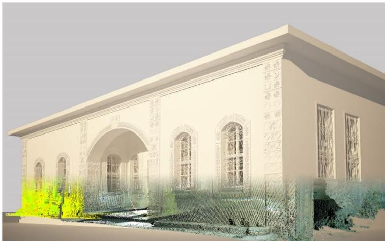
**Figure 12.** 3D Cad model of houses base on point cloud data.
