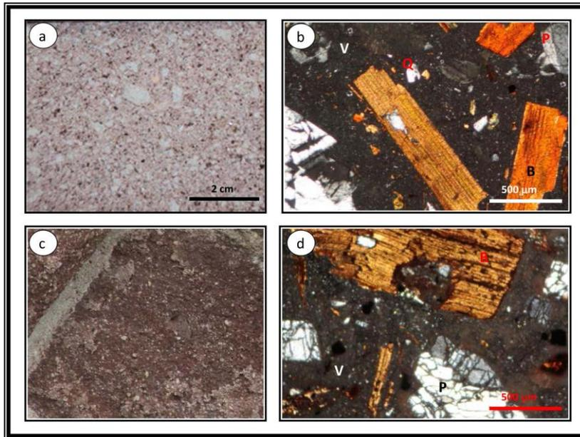
**Figure 2.** Macroscopic image of samples a) fresh, c) deterioration, microscopic image of samples b) fresh, d) deterioration (crossed polars)(P:plagioclase,B:biotite,V:volcanic glass, Q: quartzite).
