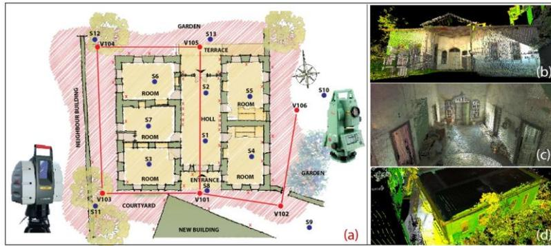
**Figure 6.** (a): Topographic network of fieldwork (b): Point cloud view of south façade. (c): Point Cloud view from inside of building. (d): Perspective view of the house.
