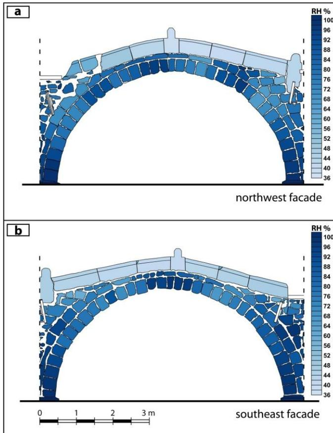
**Figure 5.** Relative humidity maps of stones in the Mısırlıoğlu Bridge, a) northwest facade, b) southeast facade.
