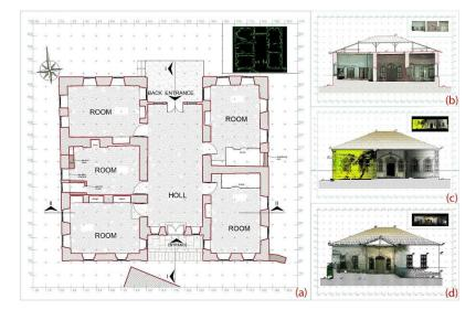
All ortho-images exported from Cyclone contain georeferences data thanks to some collateral files (TWF, TFW extensions). When these images are imported into AutoCad, thanks to some special tools, these images can be taken places according to coordinate system coming from Cyclone.
