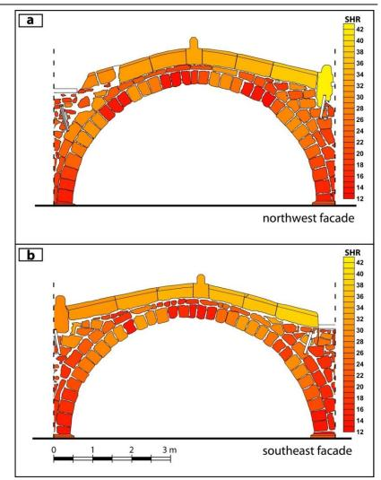
**Figure 7.** SHR distribution maps of the building stones in the Mısırlıoğlu Bridge, a) northwest facade, b) southeast facade.
