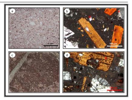
**Figure 2.** Macroscopic image of samples a) fresh, c) deterioration, microscopic image of samples b) fresh, d) deterioration (crossed polars)(P:plagioclase,B:biotite,V:vol canic glass, Q: quartzite).
