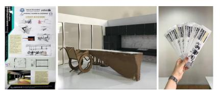
The kitchen design consists of a bench and an island module. The bottoms of all the cabinets in the bench module in front of the wall are left empty to a sufficient height at a level suitable for the knee distance on a sloping ground. This idea is an appropriate solution in terms of universal design principles. This allows the foot of the wheelchair to get down and more convenient access to the
