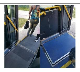
**Figure 9.** Bus ramp detail from USA (Yılmaz 2017).
