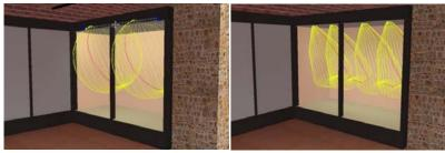
Alternative C: Horizontal linear luminaire behind the upper metal profile
